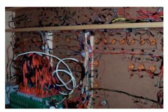
The "inputs" panel into the interlocking mechanism consist of wiring twenty (20) Turnout levers, four (4) diamond-protecting signal levers, ten (10) rotary switches, and thirty-four (34) push buttons, one for each of the previously mentioned items. "Outputs" consist of over 200 LEDS on the Panel Track Diagram for reporting block occupancy as well as turnout, signal, and traffic request lever positions.
